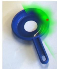
(b) Constrained grasp density (green) and optimal grasp position (red)
