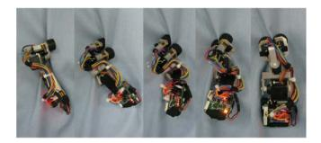
Fig. 14. The performance on recovery from the side tumbling
