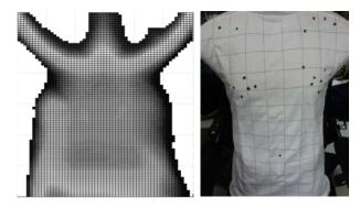
Fig. 11. Comparison between the model and the actual unreachable area: the black points on the clothes in the right figure are the recorded points where the robot cannot climb, while the white area in the left figure is the theoretical unreachable region. They have the similar shape on the clothes.
