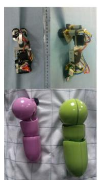
Fig. 1. Prototype and the improved visions of Clothbot: the upper figures are the prototype of Clothbot and the lower robots are the improved Clothbots, which are equipped with protective shells.
