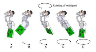
Fig. 10. Tail's motion to recover from a side tumbling
