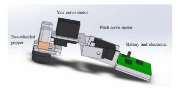
Fig. 2. Structure of Clothbot: Clothbot is composed of a two-wheeled gripper and a 2-DOF tail. The tail consists of the yaw and pitch servo motors. The battery and electronic are fixed at the end of the tail.
