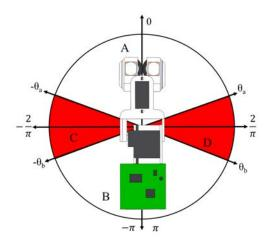
Fig. 8. Analysis of the direction of Clothbot: the white/red area indicates the feasible/infeasible direction of movement.
