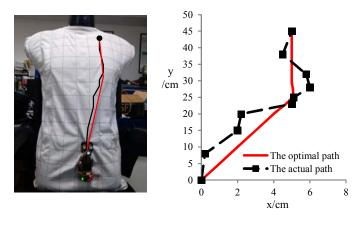
Fig. 13. Comparison between the optimal and the actual path in the test
