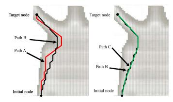
Fig. 9. The comparison between the path of  $A^*$  algorithm and the improved  $A^*$  algorithm: Path A is the path of the  $A^*$  algorithm while Path B is the path of the improved  $A^*$  algorithm with the weight of the locomotion, respectively. Path C is the smoothed path.
