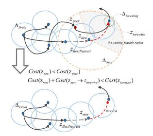
Fig. 2. Drain and Rewiring method after generating a new node is graphically presented in a selected picture.
