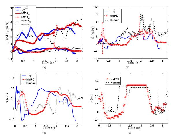
Fig. 6. Experimental comparison results under the autonomous controller and the human expert driver. (a) Vehicle velocity profiles. (b) Yaw-Rate ( $\dot{\psi}$ ) profiles. (c) The body center slip angle ( $\beta$ ) profiles. (d) Steering angle ( $\delta$ ) profiles.
