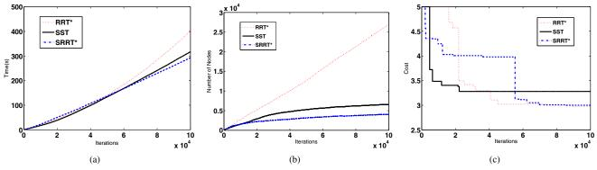
Fig. 3. Comparing the number of the nodes, computational time and convergence of the cost function for vehicle motion planning. (a) The elapsed time of different methods for the car mode. (b) Number of the generated nodes for the car model. (c) Convergence of the cost function (Time) for the car model.
