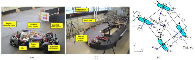
Fig. 1. (a) Autonomous scaled vehicle. (b) The indoor robotic vehicle testing track. (c) A schematic of the robotic vehicle motion.
