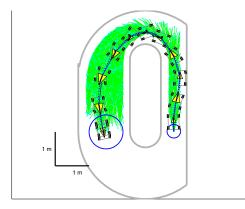
Fig. 4. The time-optimal trajectory using the Sparse-RRT\*. The results are obtained under 500,000 iterations, 2,573 nodes, 1,570 rewiring and 601,260 of drained nodes in 1,063.97 seconds. ( $\Delta_{\text{Near}}=0.5$  and  $\Delta_{\text{Drain}}=0.1$ ). The optimal traveling time is found as 2.93 s.
