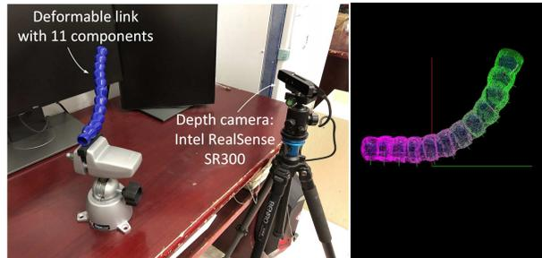
Fig. 3. Experiment devices include the deformable link with 11 components and the Intel RealSense SR300 as the depth camera.
