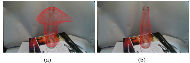
Fig. 1. Shape reconstruction results overlaid as red projected vertices on the image: (a) using a camera-only method and (b) our sensor fusion method.
