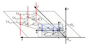
Figure 2: Superimposed CCSs x - y - z and ICSs u - v for the vertical line i over frames k - 1, k and k + 1.
