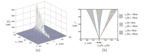
**Fig. 3.** (a) An illustration of  $|e_{\Delta}|$ . Robot positions are set to be  $x_w(0) = 10$  cm,  $z_w(0) = -50$  cm. (b)  $A_u$ s with different robot positions  $(x_w(0), z_w(0))$ , which are the black dots in the figure. We set the threshold  $e_t = 0.2z_w$ .
