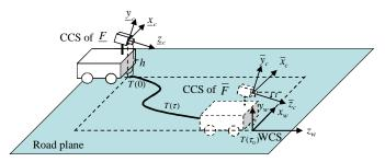
Fig. 1. Definition of coordinate systems and their relationship. The WCS is a fixed coordinate system while a CCS is attached to the moving camera.
