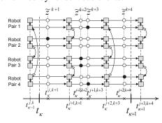
Fig. 1. A sample information flow graph for four robot pairs. Gray rectangles represent robot rendezvous events. Arc arrows in vertical direction indicate information exchange between robots in communication range. Black and white circles represent events for robots with and without detection of active radio transmissions, respectively.
