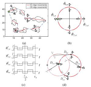
Fig. 2. Sample results for the decentralized planning using 4 robot pairs. (a) Sample robot trajectories of DPRWA. The solid red and dashed blue lines represent the on-ridge and off-ridge movements, respectively. (b) An example of the intra-ring movements on the time ring. (c) Changes of robot pair directions corresponding to the intra-ring movements. (d) Sample interring movements using time ring space instead of Euclidean space.
