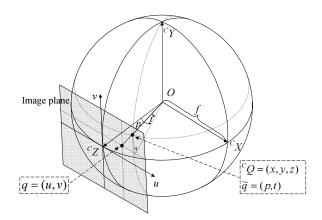
Fig. 2. An illustration of spherical pre-projection and coordinate systems: q in image coordinate system,  $\tilde{q}$  on the local spherical coordinate system, and  $^{C}Q$  is the same point as  $\tilde{q}$  but in the camera coordinate system.
