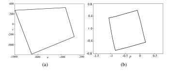
Fig. 3. Comparison of image distortion caused by the re-projection operation (a) in the original image space and (b) on the spherical surface. In this example, we perform perspective projection computation to map a rectangular image to another new location that shares  $30^{\circ}$  tilt value and has  $30^{\circ}$  pan difference.
