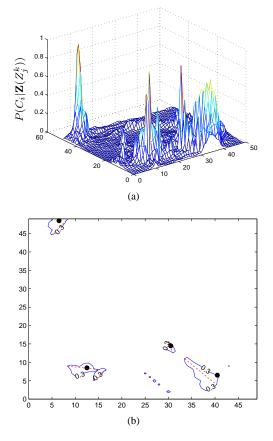
Fig. 5. (a) An example of  $P(C_i|\mathbf{Z}(Z_j^k))$  distribution, (b) Radio source locations, a sample level set L(0.3), and ridges over a  $50 \times 50$  grid for the case. The radio source locations are shown in black dots. Level set is bounded inside the blue solid lines. The red dashed lines are the corresponding ridges for the level set components.
