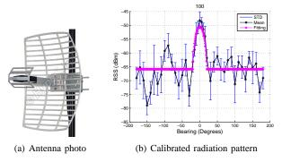
Fig. 3. HyperGain HG2415G parabolic directional antenna properties.
